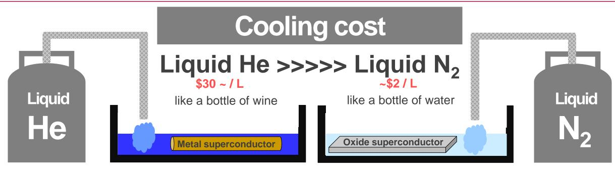
Superconducting state using liquid nitrogen cooling, which is much more low cost than liquid helium, has become possible!!
