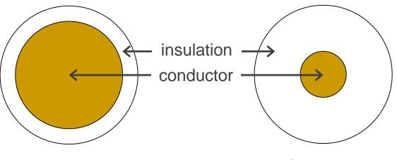
Increase cross-sectional area of conductor (higher current)
