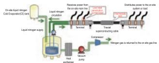
11 kV class triaxial superconducting cable system applicable to in-plant power distribution
