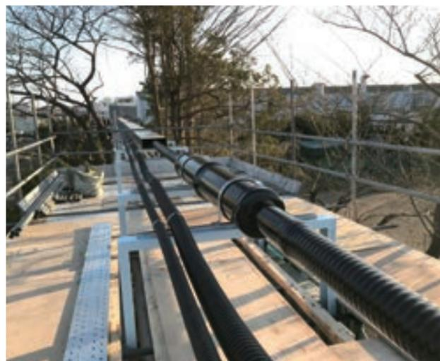
Tri-axial superconducting cable system proof of concept
