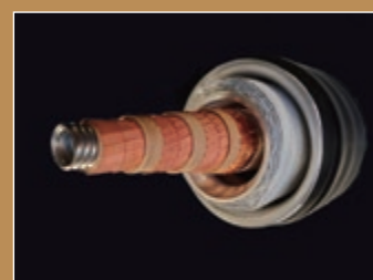
Three-phase coaxial superconducting cable system
